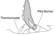
Figure 18 - Incorrect Pilot Flame Pattern
